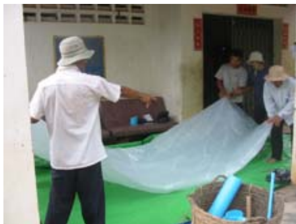
Fig 17: Folding gas reservoir
